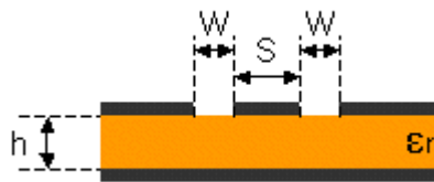
Figure 3-11 Parameters of Coplanar Waveguide with Ground 1
